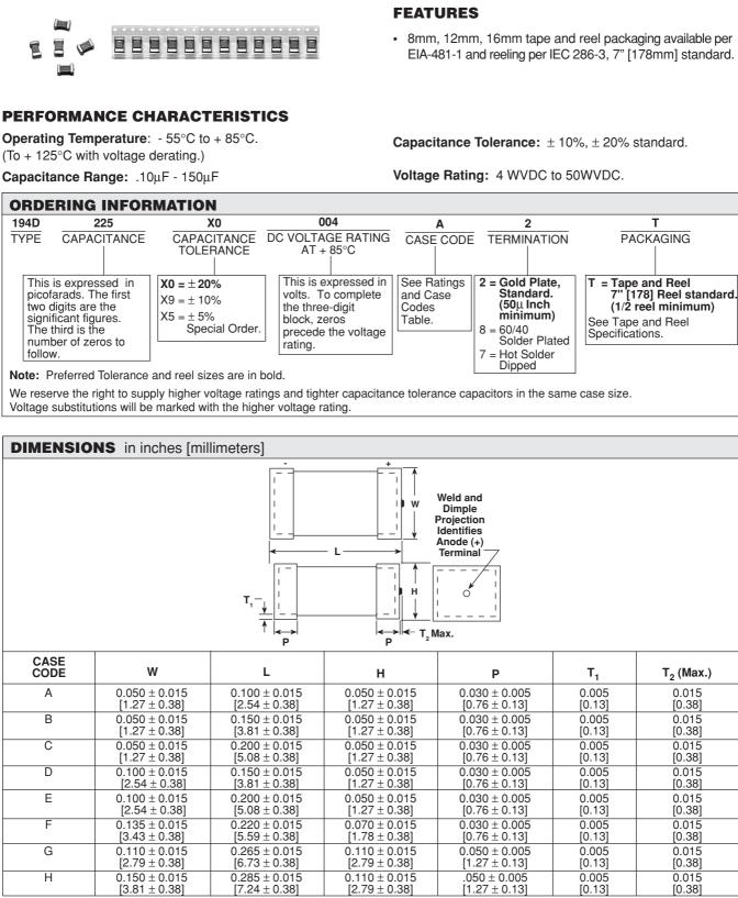
Solid Tantalum Chip Capacitors **MIDGET<sup>®</sup> Conformal Coated**
